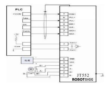
when PLC control, multiple wiring diagram
