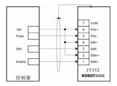
control signal +5 V anode single-ended wiring diagram
