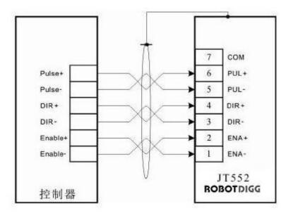
control signal wiring diagram
